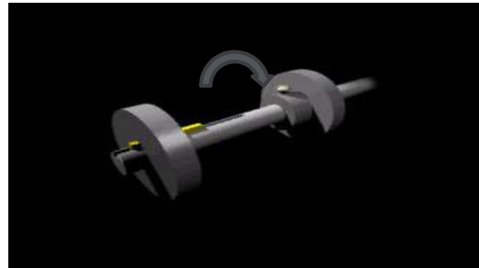
Rotating Shaft and Pulleys with Projecting Key and Set Screw
