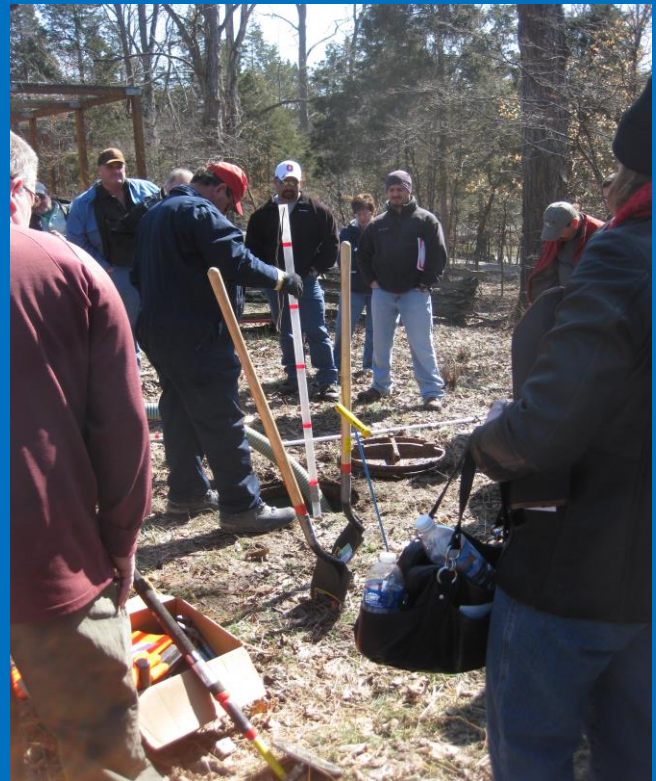
Tom Frank uses a sludge judge to evaluate the depth of sludge in a tank at Camp Camby 2013.
