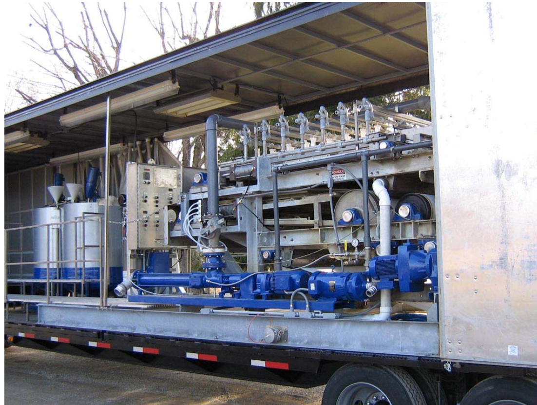
Komline Sanderson Belt Filter Press Rented to a Grease Processing Facility
